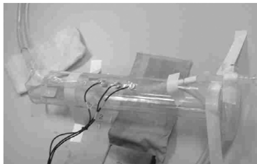
Fig.9 A photograph of the pressure sensors for Pulse diagnosis and model circulation of a radial artery
